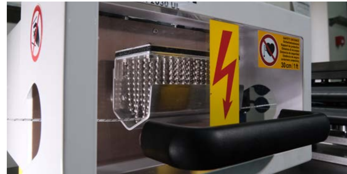
SPARK TEST %100 isolation control and verification
