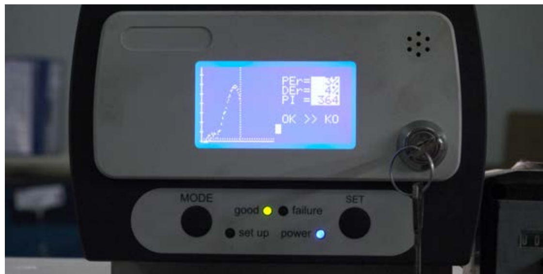
CRIMP FORCE TEST %100 crimp force measurement control Automatically stops when crimp force exceeds the given range
