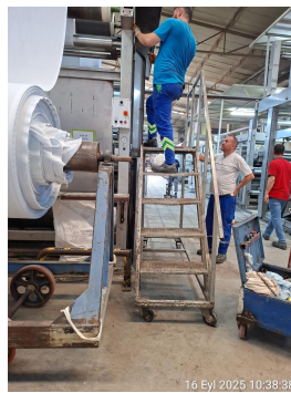
NC-Unsafe Working on Moving High Platform_No Break on Wheels.jpg
