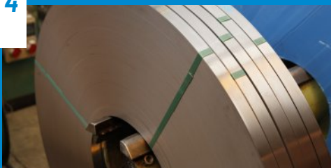
Slitted coils, properly wrapped and strapped at the final stage and made ready for packaging.
