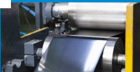
The material surface quality, tensile strength and mechanical homogeneity increases after rolling.
