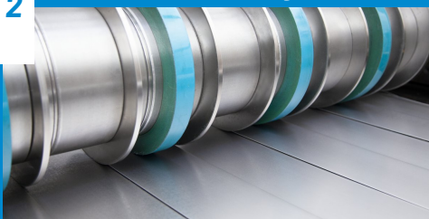
Cold rolled coils are brought to desired widths by slitting clean and burr-free in our slitting machines.
