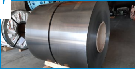
Cold rolled coils as raw material.
