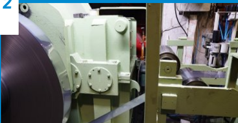
Sheet thicknesses are rolled within the precision thickness tolerance by between 0.30-3.00mm.
