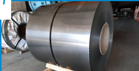
Cold rolled coils as raw material.
