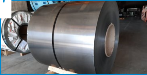
Cold rolled coils as raw material.
