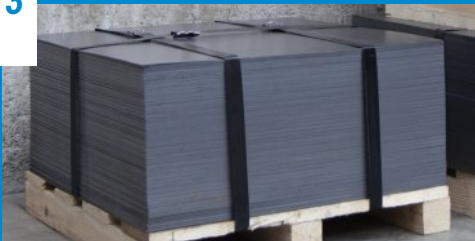
Sheets that are cut to length are arranged properly and strapped and prepared for shipment.
