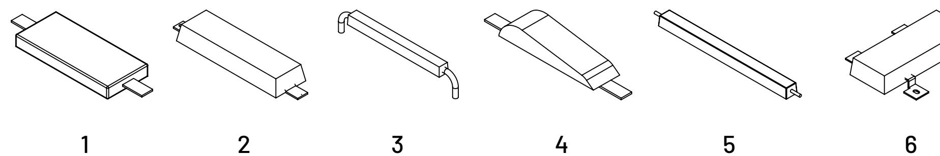
**SOME ALUMINUM ANODE DIMENSIONS USED ON SHIPS ARE GIVEN BELOW.**
