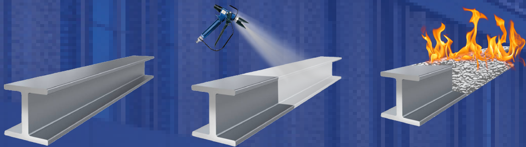
Steel Protected with Fire Retardant Coating
