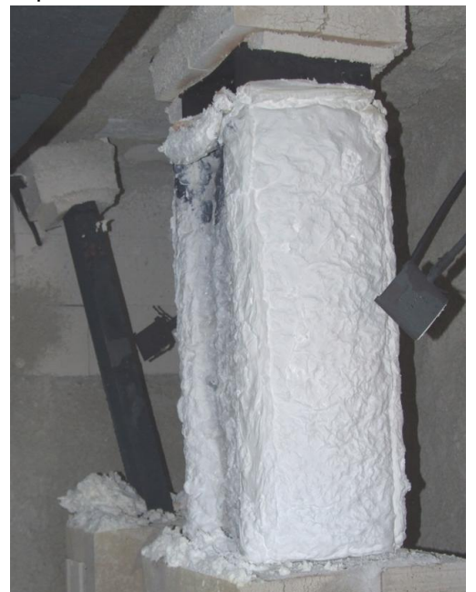
Specimen No. 15SC and 21SC after the test
